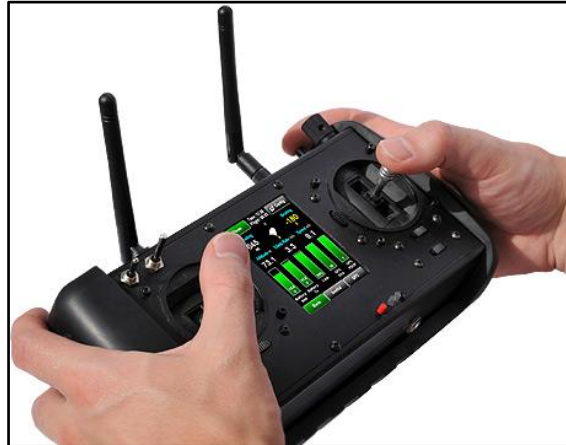
Figure 2.2. The Draganflyer X6 handheld controller (Draganfly Innovations Inc. 2013).
