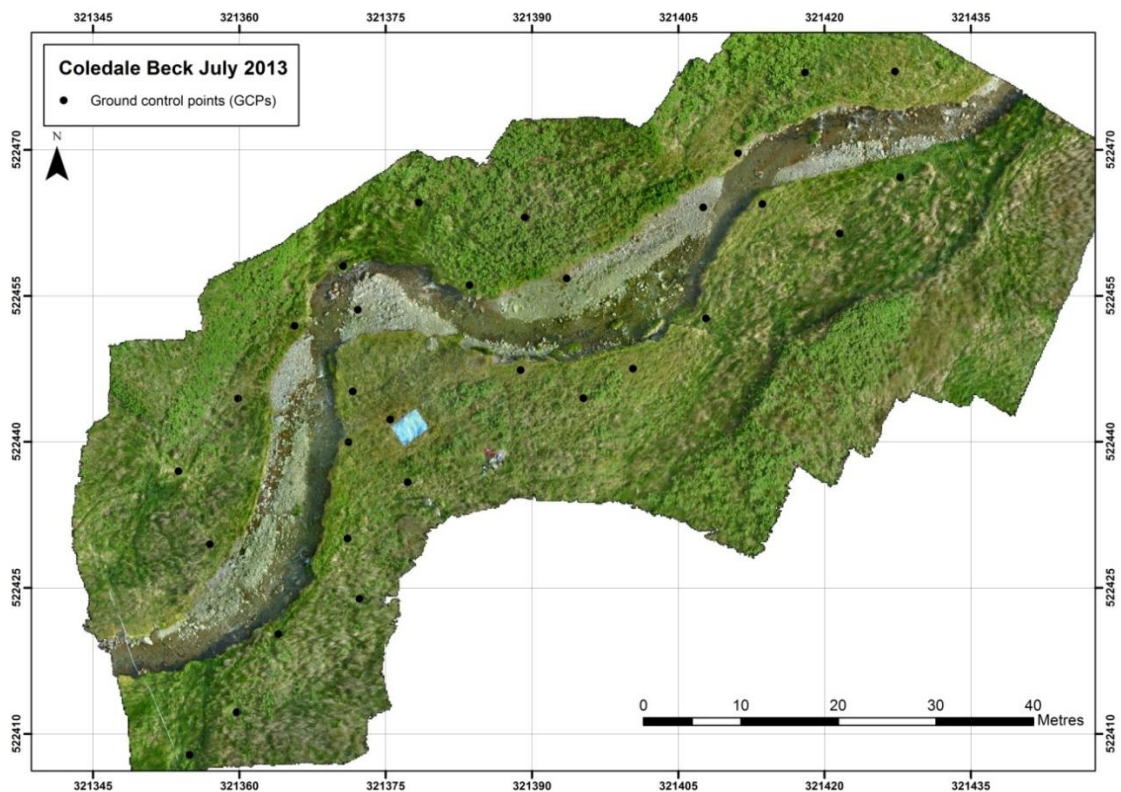
Figure 2.12. Locations of ground control points during the UAS survey of Coledale Beck, July 2013 (modified from Woodget et al., 2015).
