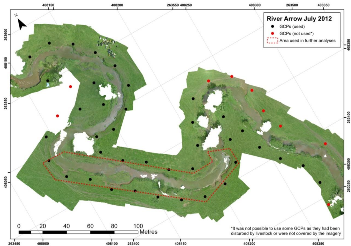
Figure 2.10. Locations of ground control points during the UAS survey of the River Arrow, July 2012 (Zone A in Figure 1.6).
