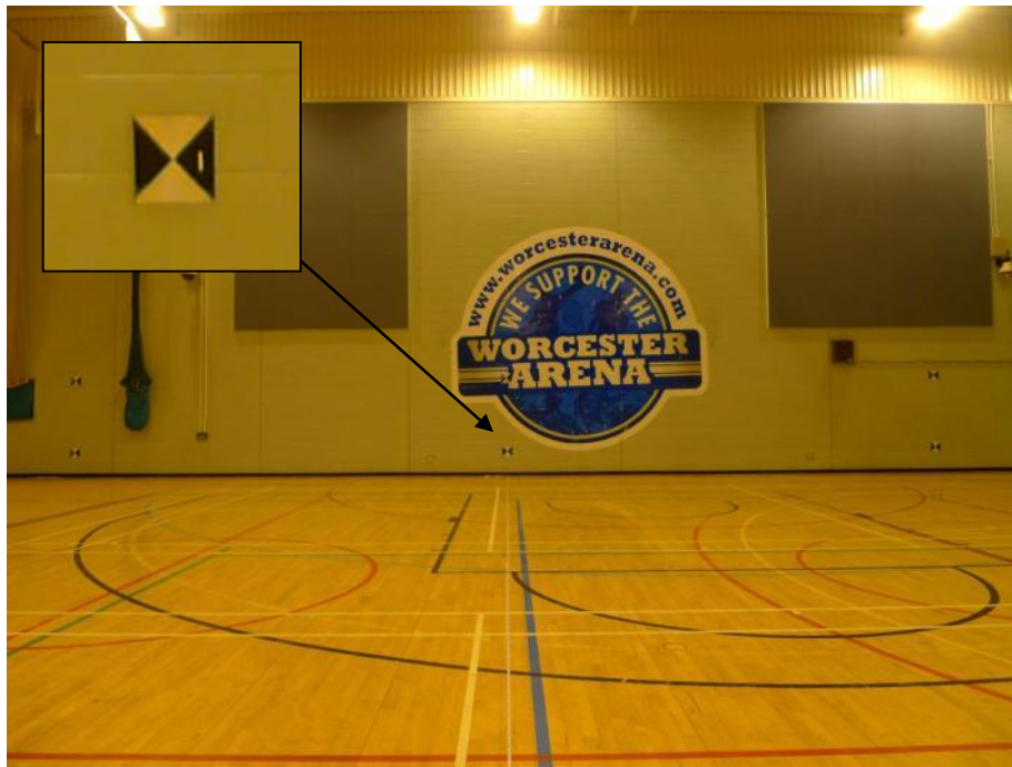
Figure 2.5. Set-up of the camera characterisation tests, with example artificial target (measuring 20cm x 20cm).
