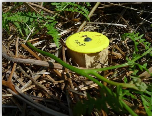
Figure 2.21. Example of a marker established at Coledale Beck and used as TLS reflective target position markers and TLS scan station position markers.
