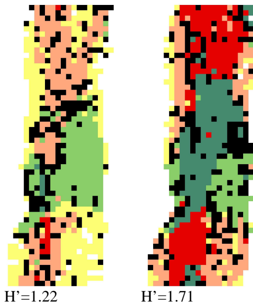
Figure 4.1 Example reachscapes with relatively low (left) and high (right) hydraulic patch diversity ( H' ).
