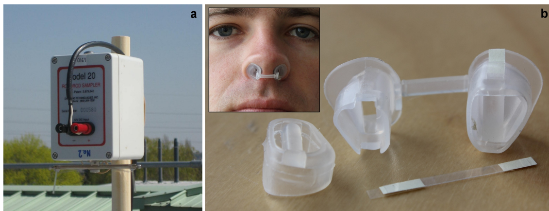
Figure A.2: The Sampling Technologies Model 20 Rotorod Sampler (a) and Model 1 Nasal Air Sampler (b).
