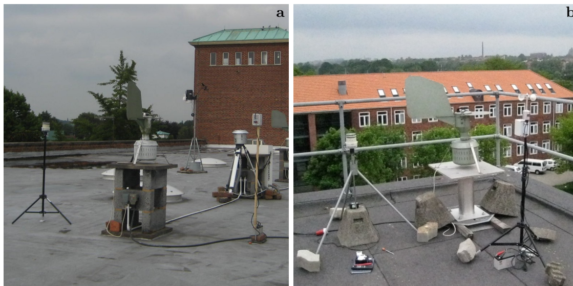
Figure 2.1: Data collection at the University of Worcester (a) and Danish Meteorological Institute (b). In both cases the PVAS stands on the right, the 7-Day sampler in the centre and the Rotorod on the left.
