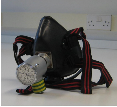
Figure E.1: Device used for estimating breathing rate during exposure sample collection - a Wright Respirometer (British oxygen type P.M., Ferraris Development & Engineering) attached to an anaesthetic mask.
