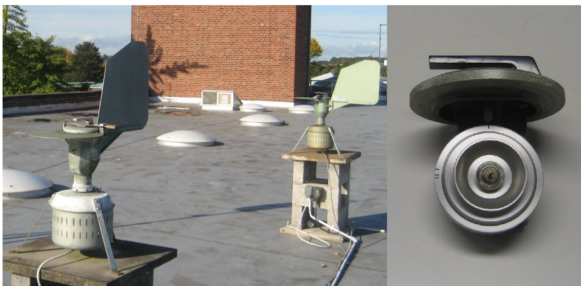
Figure A.1: Burkard 7-Day Recording Spore Trap (left) and 7-day lid assembly (right).
