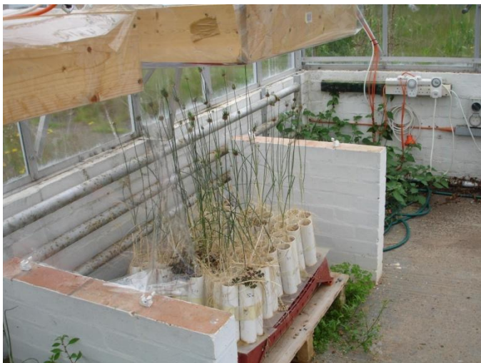
Plate 3. Experimental lighting arrays showing arrays made from a total of seven short lengths of drainage pipe glued together.
