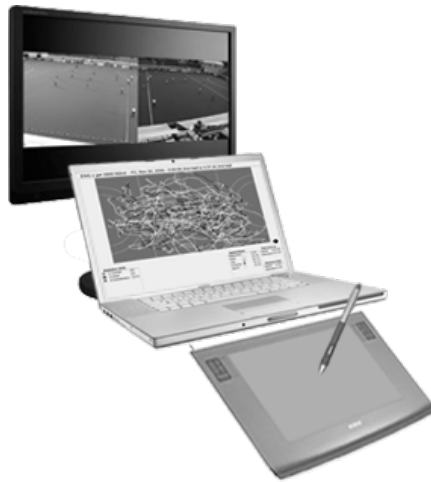
Figure 1. Set-up of computer-based tracking system TP, monitor and tablet input device.
