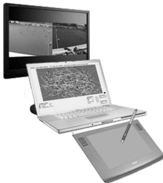
Figure 7. Set-up of computer-based tracking system TP, monitor and tablet input device.
