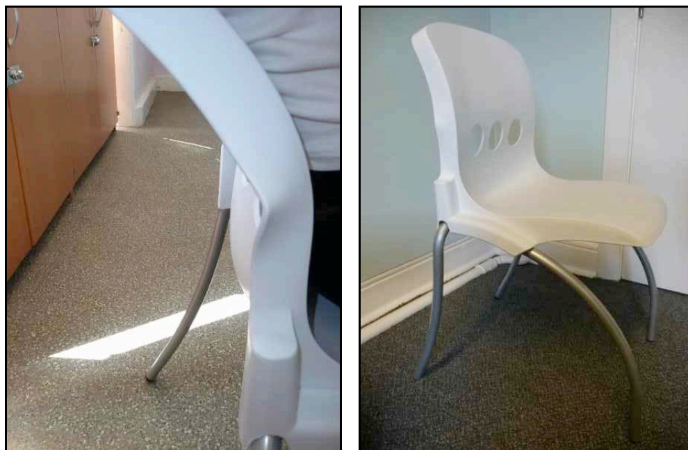
Figure 10.9: The flexible back of the chair bending when a student leans back and the resulting stress point on the chair
