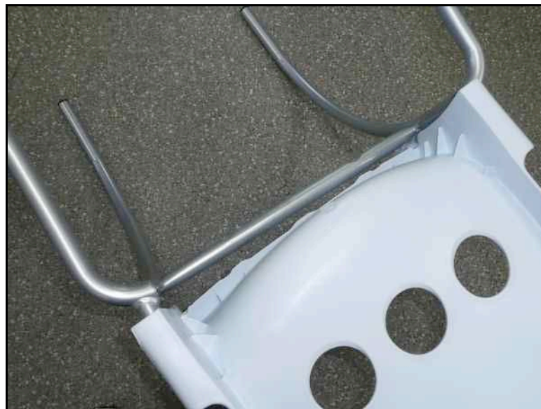
Figure 10.8: Max chair falling apart due to manufacturing errors
